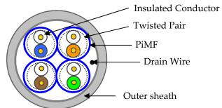
Fig 1. Cross Sectional Diagram of Cable
