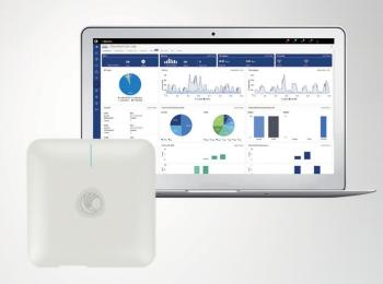
Stay on top of the latest standards with the high-powered, Gigabit speed, beamforming, Multi-user MIMO (MU-MIMO) 802.11ac wave 2 e600 access point with a 4x4 antenna array. From the classroom to the mall, cnPilot ™ e600 Indoor is perfect for applications that demand high capacity, range, and/or support high user density.
